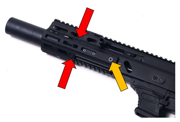
9. <u>Fastening the rail continued</u>: Tighten the rear most M-Lok mounting screws. Be sure the M-Lok T-Nuts have rotated correctly and are secured behind the M-Lok slots inside the receiver. Tighten to 30in/lb. Be sure you cannot pull up on the rail's ears to avoid snagging.
