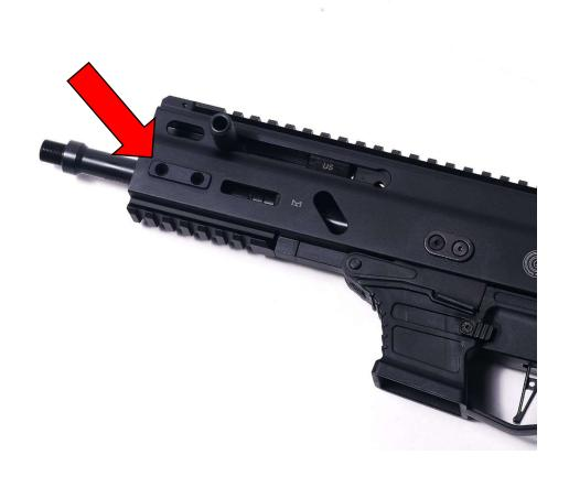
4. <u>Insert the Bridge into the front of the Receiver</u>: Apply a small amount of gun lube to the long bridge taps then insert the Bridge into the front of the receiver. The two long sides on the Bridge will be oriented side by side at the 3 and 9 o'clock positions. Be sure the Bridge is complete inserted and sitting flush with the front of the receiver. *The Bridge will not insert, if not oriented correctly.*
