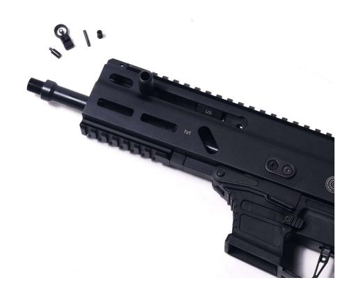
3. <u>Install Clamps</u>: Press the Clamps firmly into the 'forward most' M-Lok slot on the left and right sides of the receiver. Both Clamps should sit complete flush, flat, and even on the receiver. You may need to gently tap them into place.
